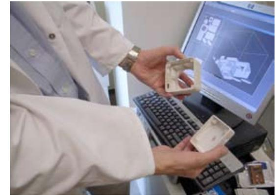
Fig. 5.15 Printed parts shown alongside CAD models
