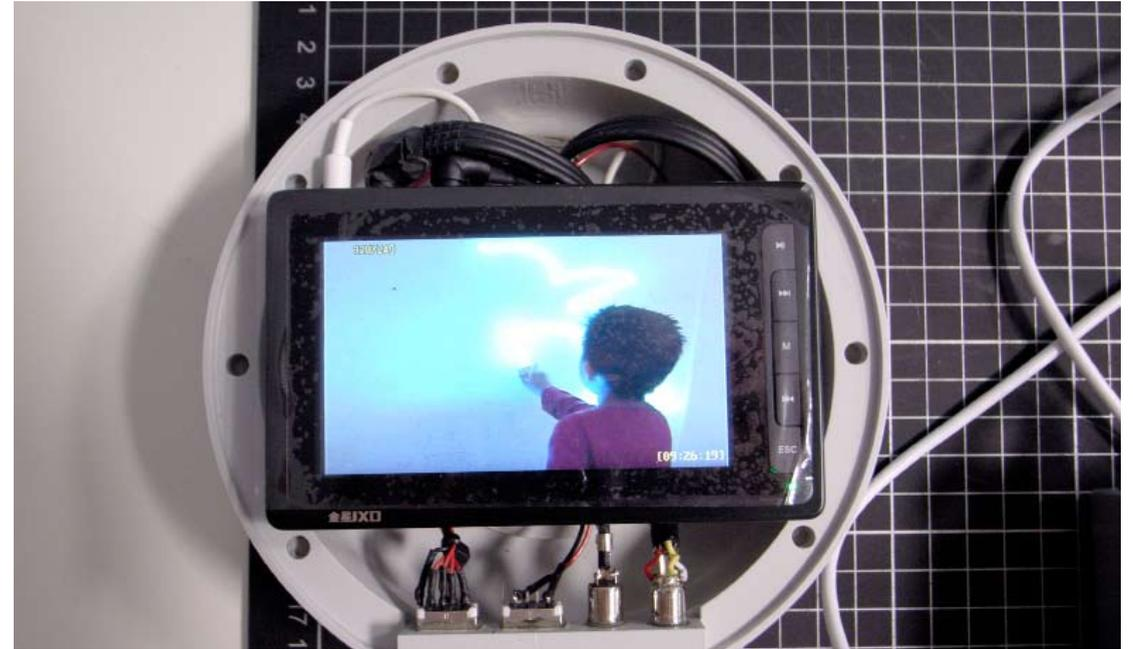
Fig. 5.24 The Neuroscope fitted with screen
